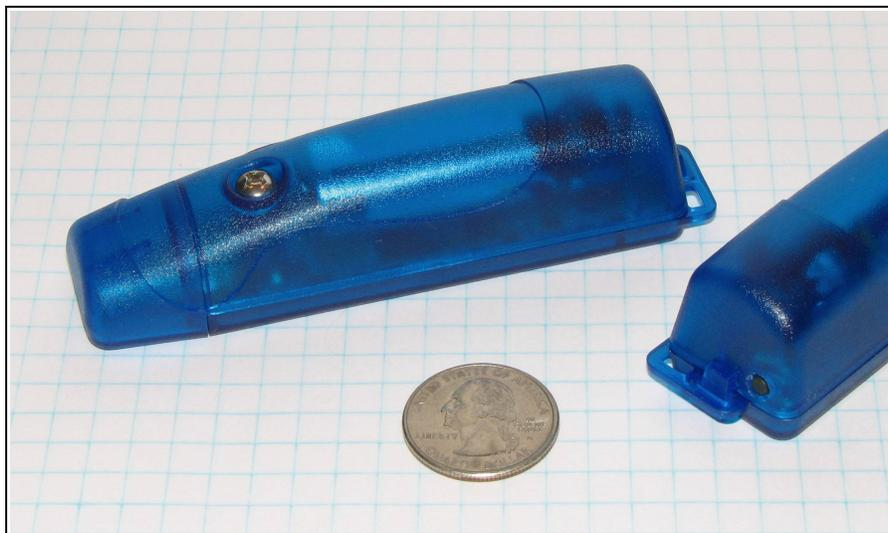
Figure 1: USB Accelerometer X6-1A
