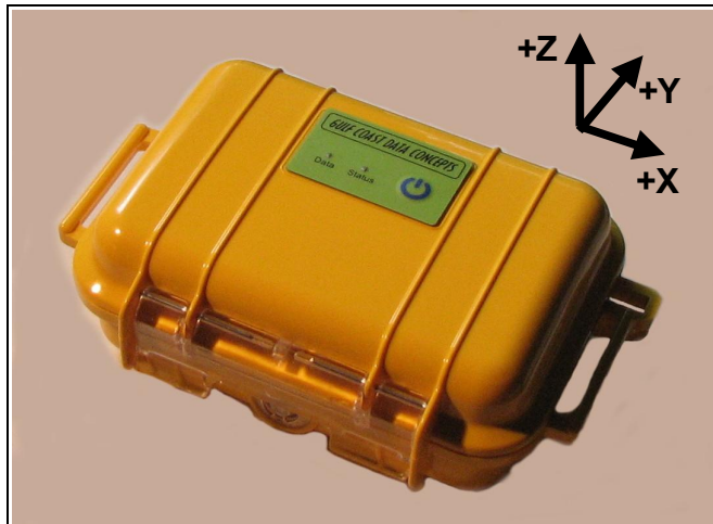
Figure 3: MEL-x2 Sensor Orientation
