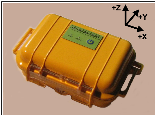
Figure 2: MEL-x16 Sensor Orientation
