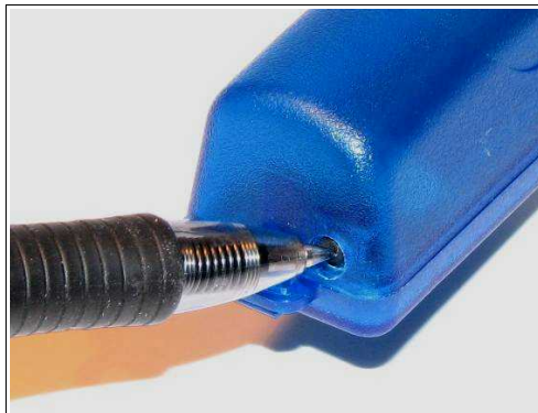
Figure 2: Starting the Data Logger
